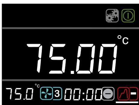
1. Rotate the dial until the **program** icon is highlighted, press the **S** button.
