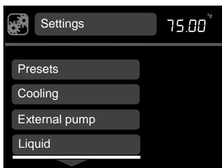
2. Rotate the dial to scroll up and down the list until **liquid** is highlighted, press **S** to select.
