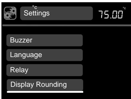
2. Rotate the dial to scroll up and down the list until **display rounding** is highlighted, press **S** to select.
