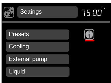
3. Rotate the dial to display preset icon 1, 2 or 3, press **S** to select.
