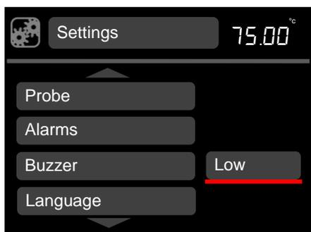
3. Rotate the dial to scroll through the volume levels (low, medium and high and off), press **S** to save the selection.
