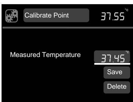
3. Rotate the dial to highlight **measured temperature**. Press **S** to select
