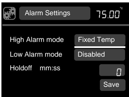
3. **High alarm mode** is highlighted, press **S** to select.
