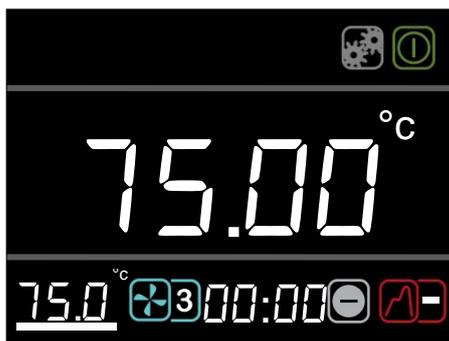
1. Rotate the dial until the **set temperature** icon is highlighted, press the **S** button.
