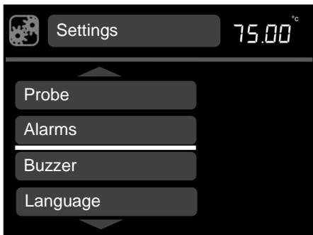
2. Rotate the dial to scroll up and down the list until **alarms** are highlighted, press **S** to select.
