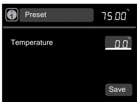
4. **Temperature** is highlighted, press the **S** button. Rotate the dial to define the temperature. Press **S** to set.
