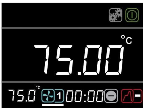
1. Rotate the dial until the **pump speed** icon is highlighted, press the **S** button.
