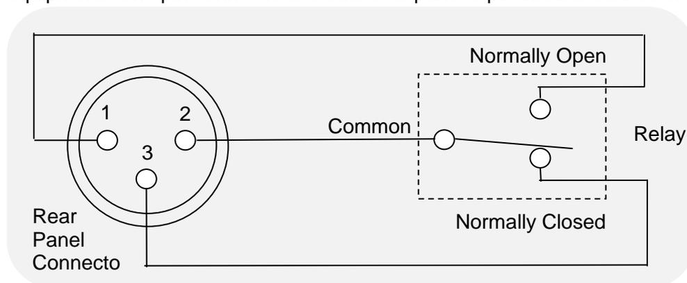
For the connecting cable use a mating XLR style connector such as the NC3FXX manufactured by Neutrik AG
