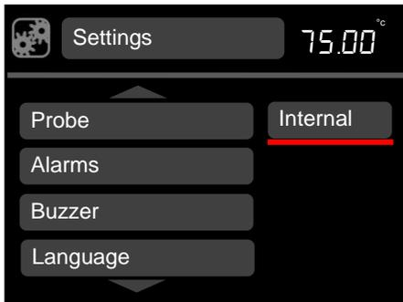
3. Rotate the dial to scroll through the probe types (**external** or **internal**), press **S** to save the selection
