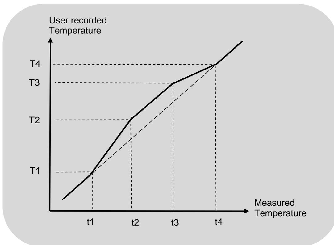
Calibration points must be a minimum of 5°C apart and there must be at least 20°C between the highest and lowest points. Any points added that do not match these criteria will not be accepted by the unit.
