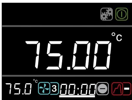
1. Rotate the dial until the **countdown timer** icon is highlighted, press the **S** button.
