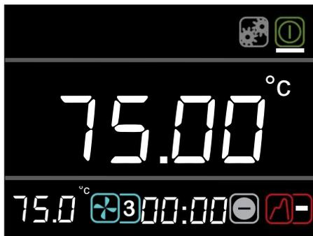
1. Rotate the dial until the **standby** icon is highlighted, press the **S** button.
