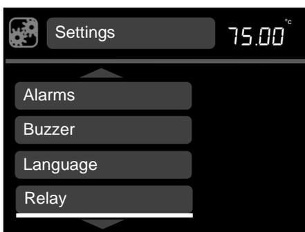
2. Rotate the dial to scroll up and down the list until **relay** is highlighted, press **S** to select.
