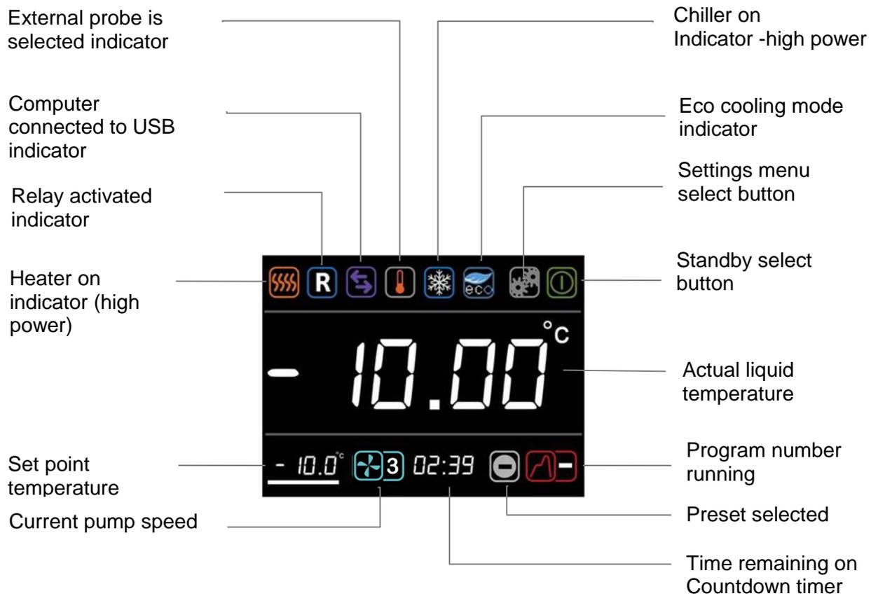
Navigation around the home screen is achieved by rotating the main dial which moves a white cursor to highlight function icons. Pressing the **S** button whilst the icon is highlighted will change the colour of the cursor to red, make the icon active and allow changes to be made, or in the case of the settings icon, further menus to be displayed. Press the **F** button to cancel an active icon. The cursor will then change to white.
