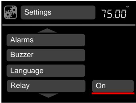
3. Rotate the dial to toggle between on/off, press **S** to save the selection.
