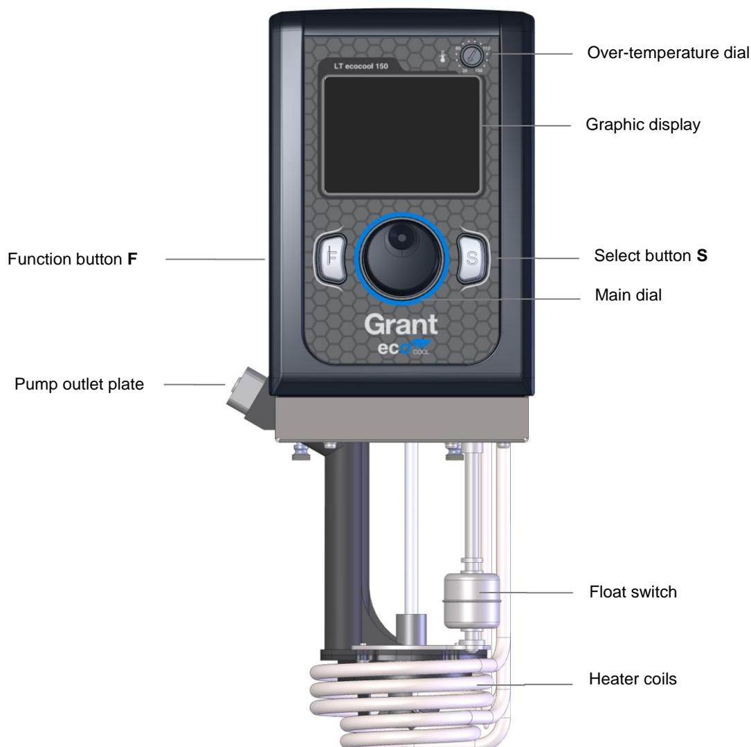
The control unit features a full colour graphic display, a main dial and two buttons F and S. All functions (setting temperature, pump speed, countdown timer, presets, programs settings and standby mode) can be configured from the home screen.
