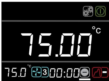
1. Rotate the dial until the **preset** icon is highlighted, press the **S** button.
